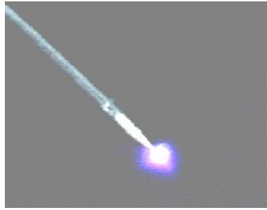
Figure showing plasma needle. The glow is cold enough to be touched
