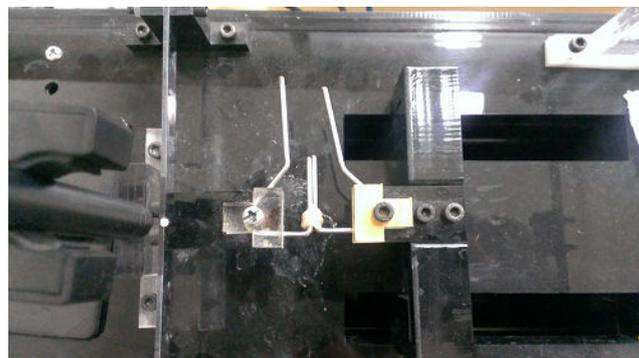
**Figure 1B.** Cervix positioned in the custom designed fixture attached to the uniaxial tensile test device, designed and fabricated to measure mechanical properties of soft biological tissues.
