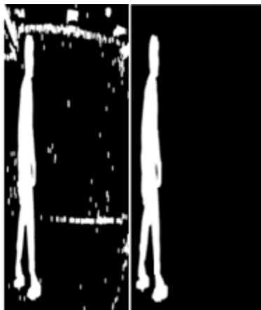
Figure 3. Background subtraction and silhouette reconstruction.
